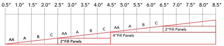
Fill Panels – ROCKWOOL Toprock DD, Toprock DD Plus or Multifix
