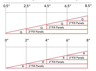
Fill Panels – ROCKWOOL Toprock DD, Toprock DD Plus or Multifix
